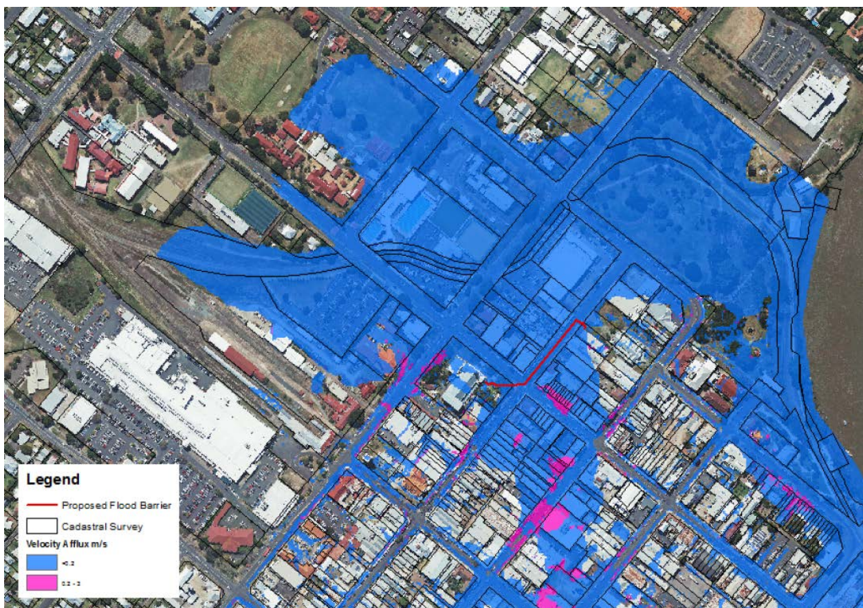
Figure A. Afflux velocity (m/s) for 100 Year ARI Design Event – Design Case
