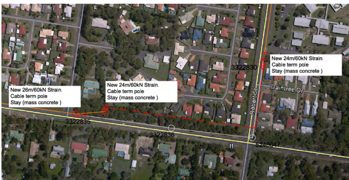
Trenching Location 60kv civil conduit
