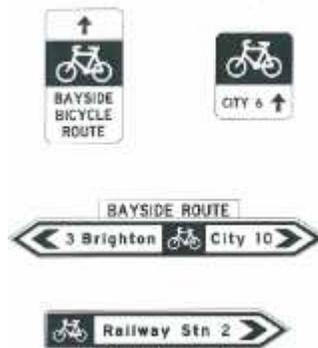
**Figure 11 – Examples of Direction Signs (Source: Queensland Manual of Uniform Traffic Control Devices)**
