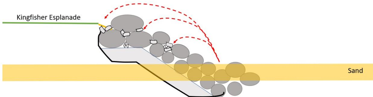
**Step 3: Wedge rock spalls into voids**
