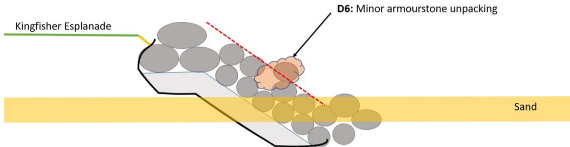
**Step 1: Identify poorly interlocked armourstone** which have wedged in armour with 3 points of contact or less and/or isolated on seawall and/or located out of slope grade and/or located near a localised void in armour
