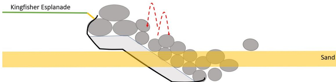
**Step 3: Wedge armourstones / increase seawall packing density locally**
