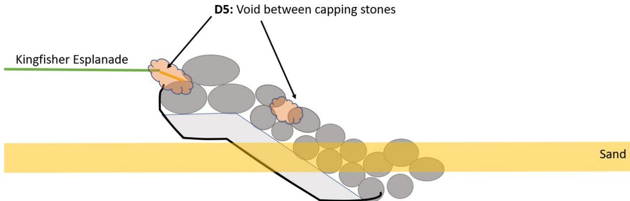
**Step 1: Identify largest voids in armourstone** which lead to
