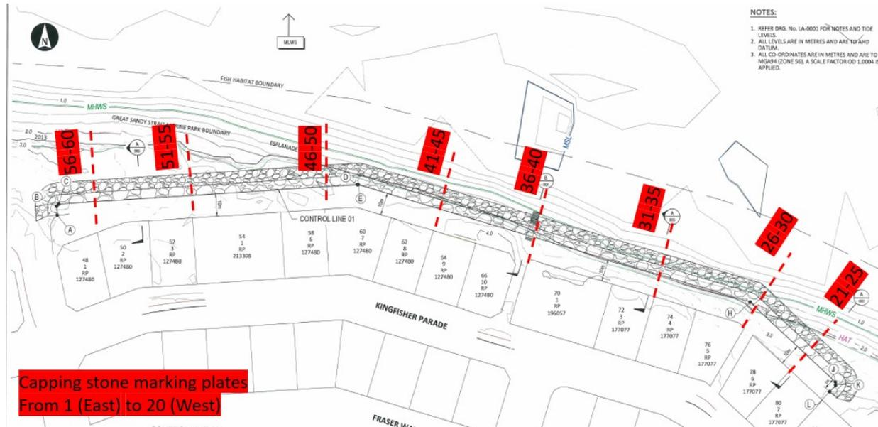
A list of visible marking plates was made during the inspection. The condition of each armourstone has been recorded. This allows to do a rapid evaluation of change to the seawall armourstone. Missing plates may be due to burial under the sand (particularly toe stones), detached plates and overturned/displaced armourstones.
