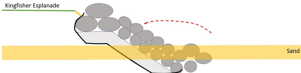
**Step 4: Re-insert the armourstone into the seawall**
