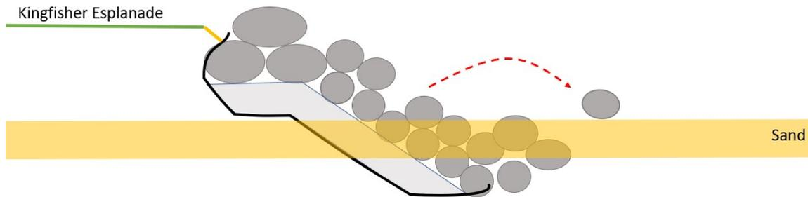
**Step 2: Remove poorly interlocked armourstone**
