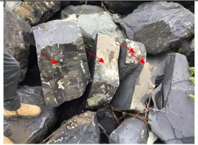
Damage 9 - multiple fractures planes and residual armourstone likely 400kg or less - #72
