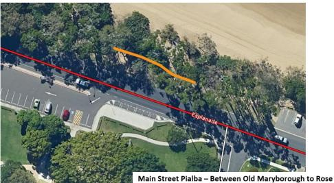
Scope: Remove and replace 40m of 3.2m wide paved footpath between various driveway accesses
