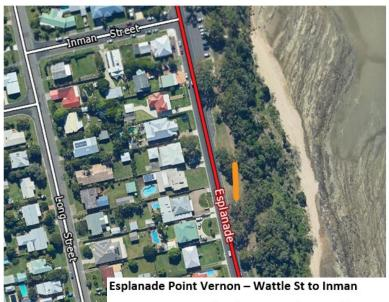
Scope: Remove and replace 89m of 2.2m wide paved footpath
