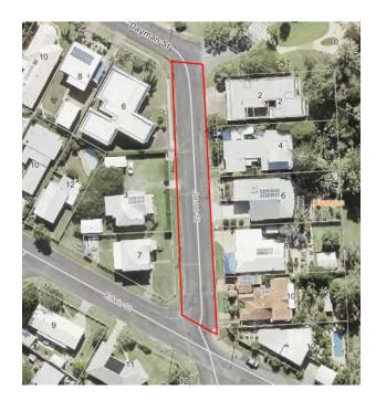
The traffic management plan that will be put in place for the duration of the construction period will allow for a one lane/one way traffic arrangement with traffic travelling in a southerly direction.
