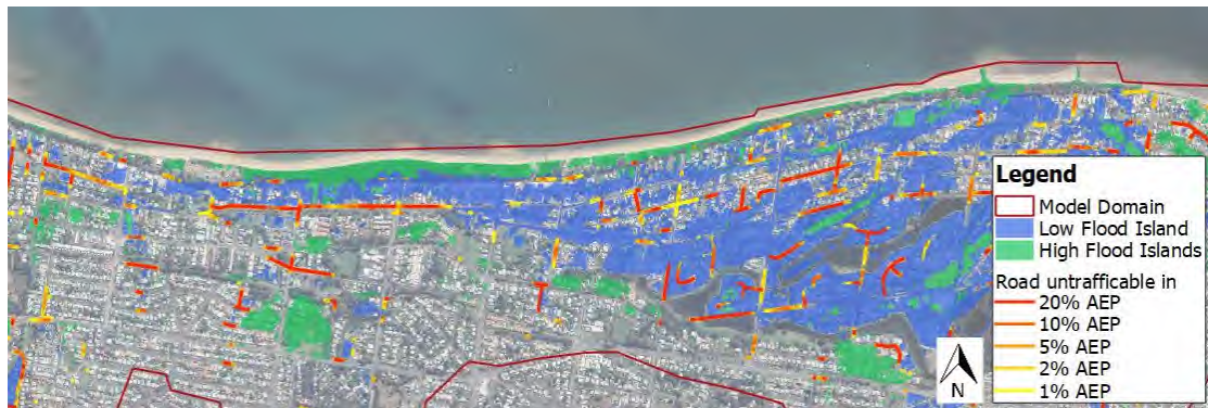
Figure 5-45 Low and High Flood Islands and Road Trafficability
