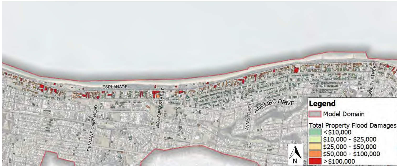
Figure 5-46 Total Property Flood Damages for the 1% AEP Storm Surge and 5% AEP Catchment Event.
