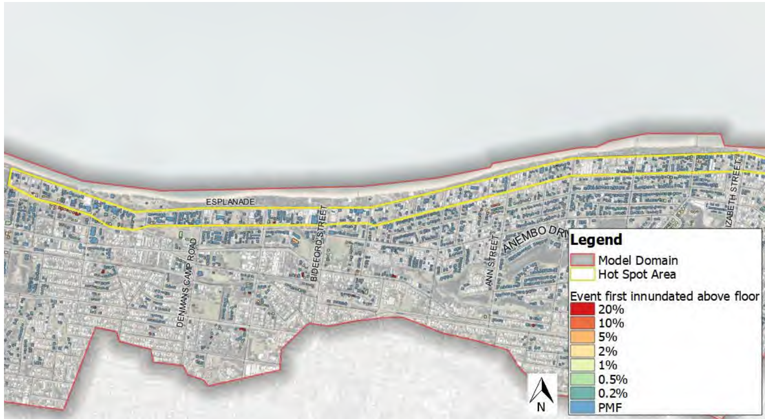
Figure 5-47 Event First Inundated Above Floor Catchment Flooding
