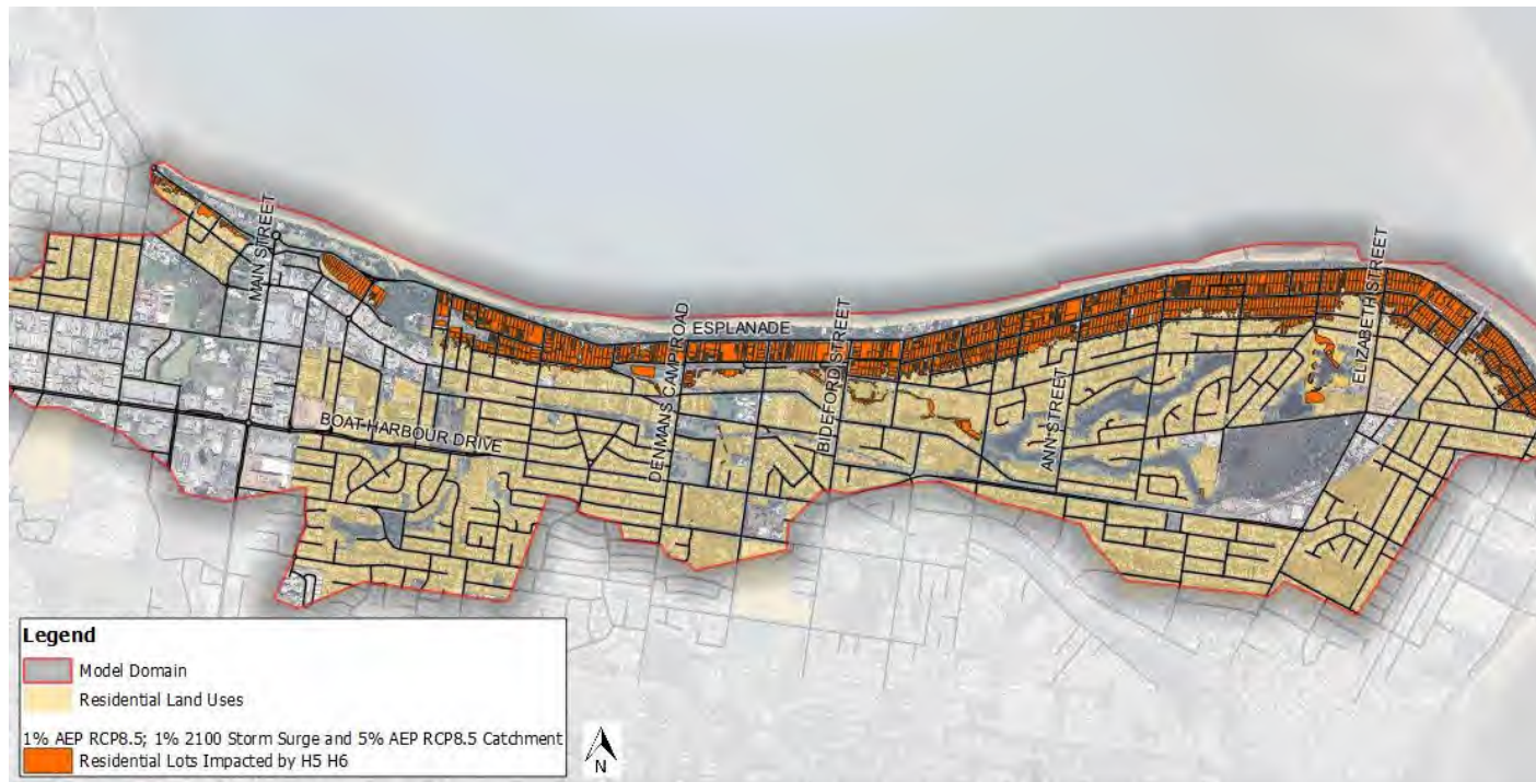
Figure 5-8 Residential Lots Exposed to H5 or H6 hazards under a Future Climate Scenario
