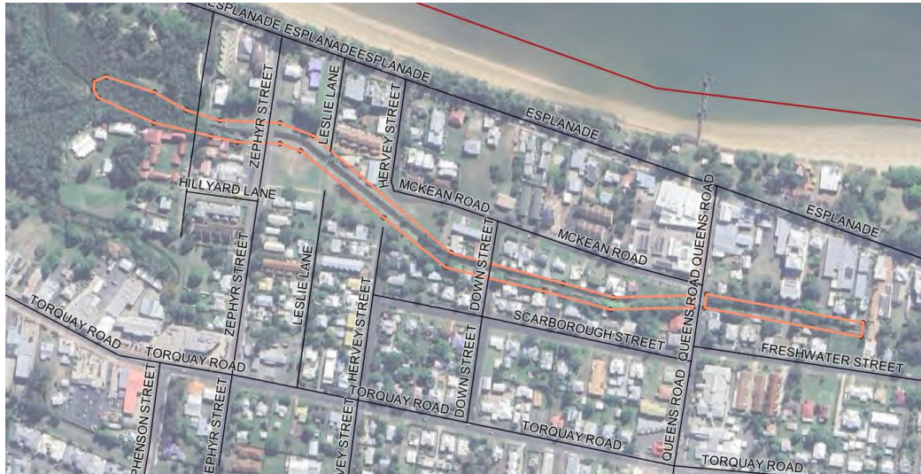
Figure 6-5 Channel widening downstream of Frank Street (MIT004)
