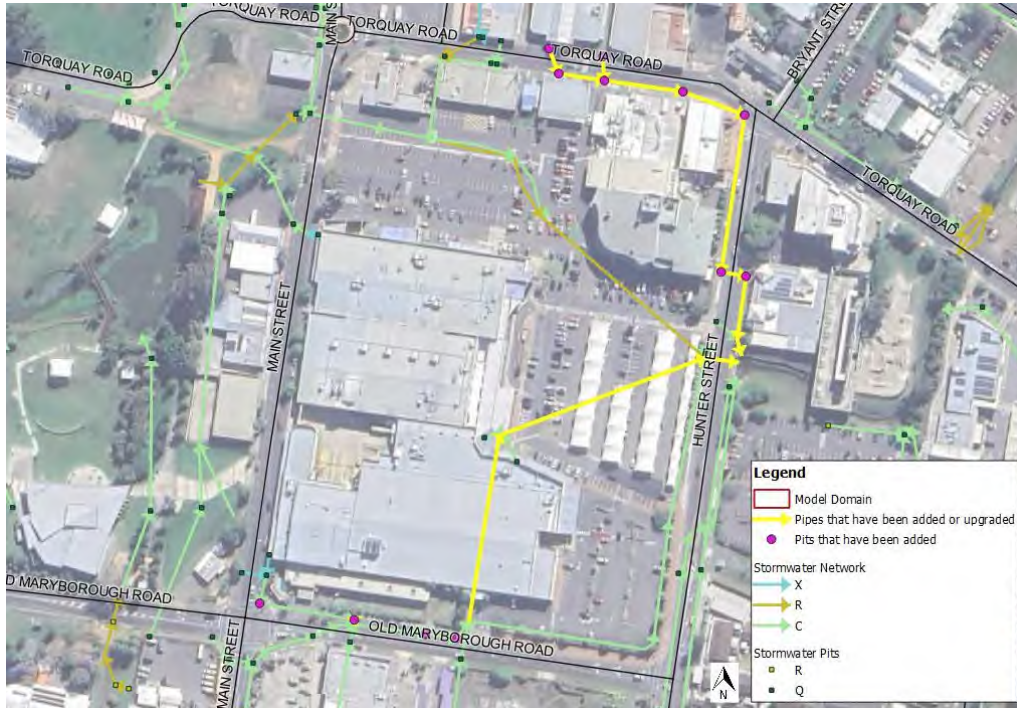
Figure 6-4 Pialba Place Drainage Improvements (MIT003)
